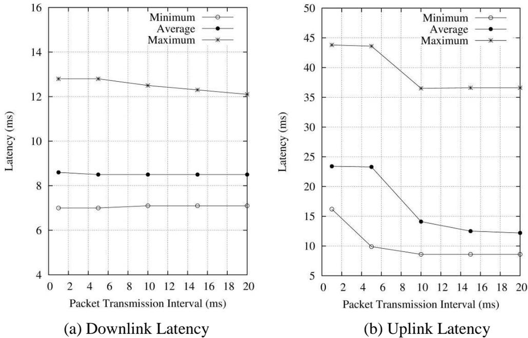
Figure 3. TD-LTE Latency vs Packet Transmission Interval
