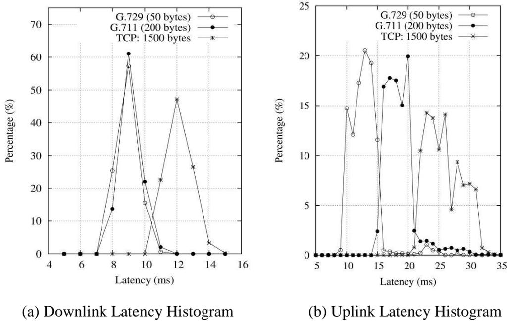
Figure 4. TD-LTE Latency Histograms for G.729, G.711, TCP Transmissions
