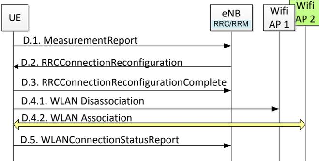
Fig. 7. Message flow for WLAN mobility.
