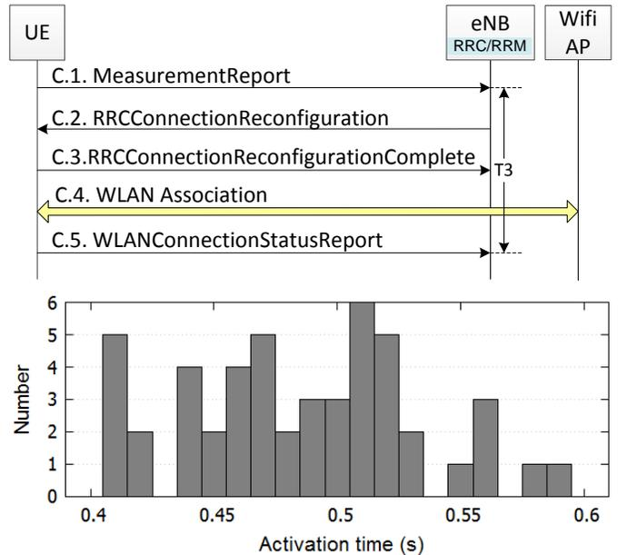
Fig. 6. Message flow for LWA activation and the T3 histogram.
