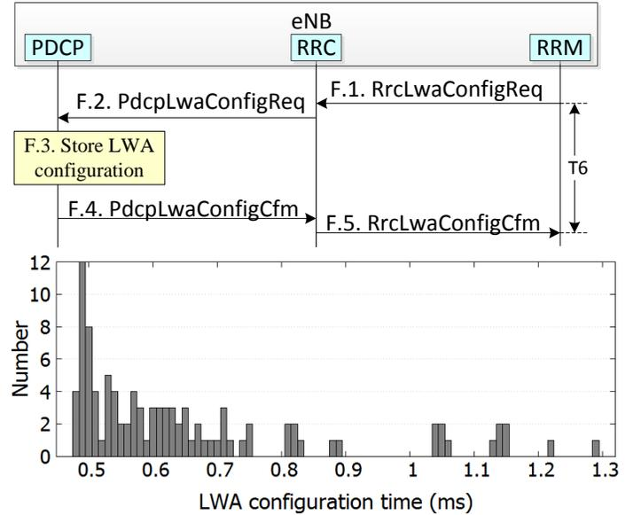
Fig. 9. The LWA configuration message flow and the histogram for T6.
