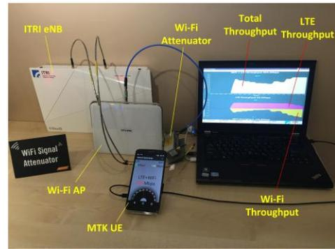
Fig. 2. The prototype of the ITRI LWA demonstrated in MWC 2016.
