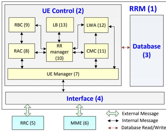
Fig. 3. Functional block diagram of ITRI's RRM.
