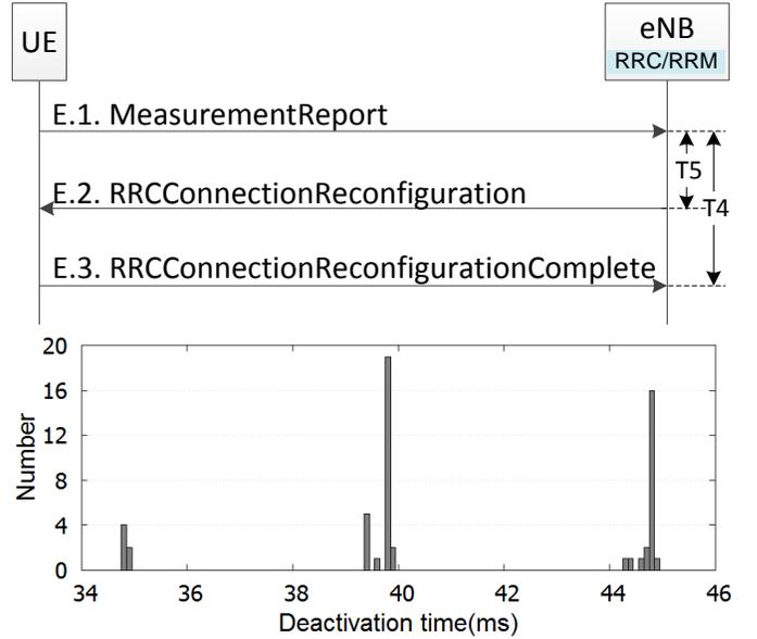
Fig. 8. Message flow for LWA deactivation and the T4 histogram.
